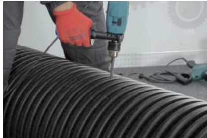
3. Drilling holes for the guided crown saw
