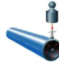
Point load test according to dr. Hassel
