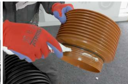
10. Lubricating appropriate connection of sag
