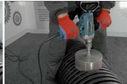
4. Drilling holes with crown saw
